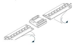
Press down on each of the pairs of connector terminals until the metal blades are flush with the top of the connector, puncturing the LED tape.
