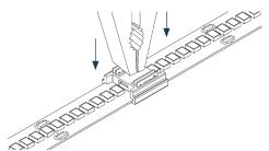
Insert Uniform LED tape into connector. (Confirm polarity of LED strips match each other)
