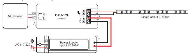
2 This product is designed with 1 DALI address input and 1 channel output, DALI address is assigned by DALI Master controller automatically, please refer to user manuals of compatible DALI Masters for specific operations.
