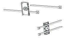
Temporarily mount the light fixture into place using the tie wraps from each concealed mount. Press all 6 nails through each concealed mount.
