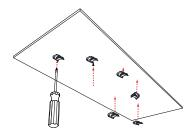
3 Slip tie wraps through both slots on the concealed mounts.
