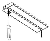
6 If jump connecting mount fixtures first then connect dimming and power jump connectors.
