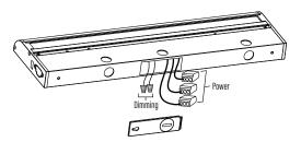
If flush connecting fixtures install dimming and power connectors first then mount fixtrue to ensure proper alingment.
