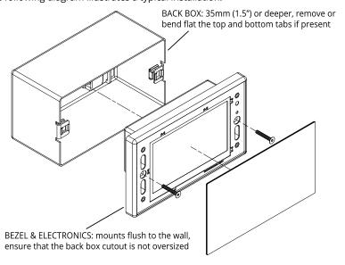
Carefully remove the protective films from the front of the liquid crystal display and the magnetic overlay before final assembly.
