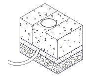
Connect Pavex lights to power leads with waterproof connectors. Place Pavex fixture in the housing ensuring that all of the cables are nested neatly in the housing unit and glass is flush with the paving stones.
