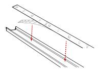
Slide grommet over power feed and run both out to channel exterior through hole drilled in step 6.
