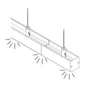
Apply light-blocking tape to the inside of all joined fixture seams to eliminate light gaps.
