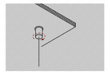
Measure ceiling and channel to determine suspension points.
