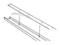
Slide grommet over power feed and run both out to channel exterior through hole drilled in step 5.
