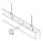
21 Cut lens to length measured in step 17.
