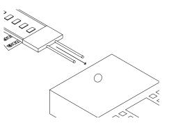
AVOID RIPPLES & OVERBENDING When removing the protective liner and applying the tape to the surface, ensure that tape is installed without any ripples or creases.
