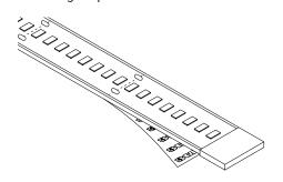
Begin peeling back protective liner to expose adhesive. Adhere LED strip to cleaned smooth, non-porous mounting surface by removing liner in short increments.
