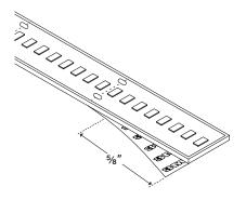
If necessary, trim OUTDOOR LED strip to desired length at indicated cut intervals. If no cutting is needed, skip to step 6.
