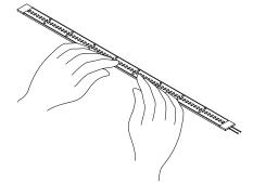
Ensure power feed on LED strip is oriented toward power source.
