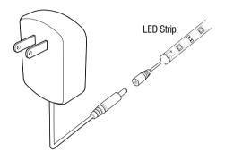
2 Plug power supply into standard electrical outlet
