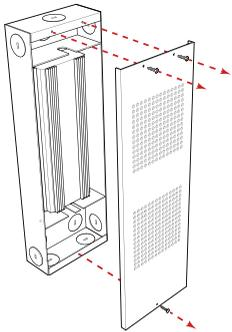
2 | Secure power supply to mounting surface.
