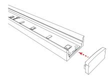
Insert channel into opening with spring clips compressed and then allow clips to release and clasp surface.
