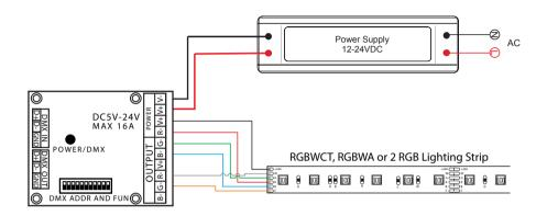
Using a small screwdriver, flip FUN switch located on the dip switch board to the "ON" position.
