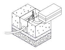
Connect the power leads to the power supply. Please refer to power supply installation instructions for further details.
