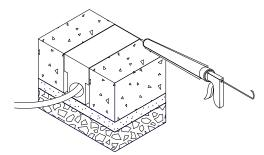
Connect Pavex lights to power leads with waterproof connectors. Place Pavex fixture in the housing ensuring that all of the cables are nested neatly in the housing unit and glass is flush with the paving stones.
