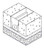
Optional step. Apply a bead of silicone between the face edge of the light source and the stainless steel housing.
