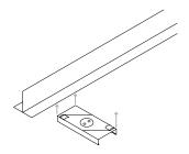
Tune the flat tile mounts counterclockwise against T-bar.
