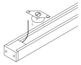
Press the top face of the drop tile mounts flush to the T-bar.
